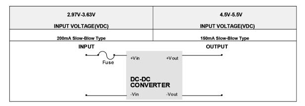
Note: Certain applications may require the installation of external fuse in front of the input.
